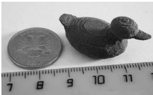
Fig. 13 Small-scale duck shape produced by SLS–SHS [176]
